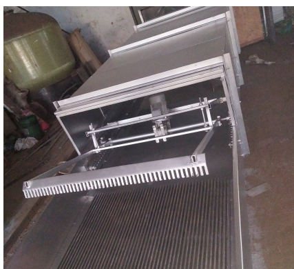
MECHANICAL BAR SCREEN
